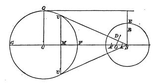
The ends of the transverse axis A, A' are the poles of the tangents at F and G;
